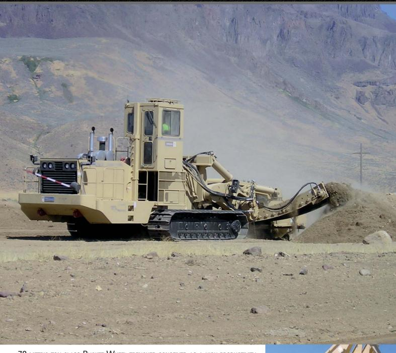
70 metric ton-class Bucket Wheel trencher conceived as a high-productivity machine for big diameter pipelines and utilities projects in dirt and light rocky soils, this model can dig up to 9'6'' (291 cm) deep and 66'' (168 cm) wide. Its buckets can be equipped with conical or spade tools to ensure the maximum productivity according to the different ground conditions.
