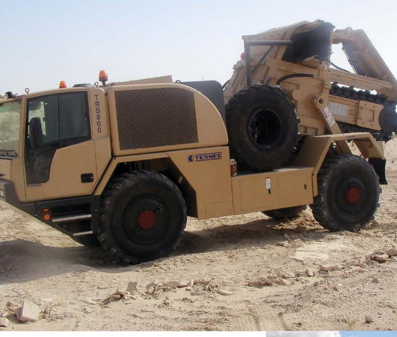
HIGH-MOBILITY OFF-ROAD TRUCK (4WD) EQUIPPED WITH BUCKET CHAIN ATTACHMENT, SPECIALLY DESIGNED TO BE EMPLOYED IN DIRT AND SOFT ROCK EXCAVATION. RADIO-REMOTE CONTROLLED MACHINE. CENTRAL TIRE INFLATION SYSTEM (CTIS) THAT PERMITS TO CONTROL TIRES PRESSURE FROM THE CAB. THE 800 CAN CUT TRENCHES UP TO  $6'\ 7''\ (200\ \text{CM})$  DEEP AND  $2'\ 11''\ (90\ \text{CM})$  WIDE.
