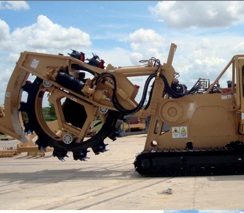
BUCKET WHEEL VERSION OF THE 775DT CS, THIS LIGHT BUCKET-TRENCHER CAN GRANT AN EVEN AN EVEN HIGHER PRODUCTIVITY IN TERMS OF METERS-YARDS PER HOUR. TRENCHTRONIC EQUIPPED, THIS MACHINE HAS BEEN SPECIALLY DEVELOPED TO BE EMPLOYED IN "DIRT" EXCAVATION; ITS COMPACT DIMENSIONS AND WEIGHT MAKE THE 775DT BW VERY EASY TO USE AND TRANSPORT.
