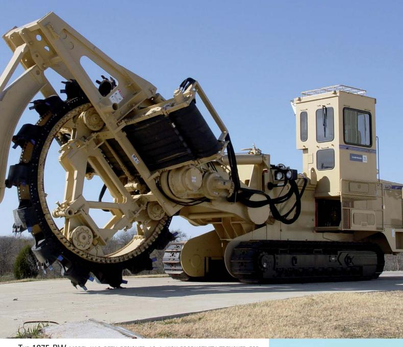
THE 1075 BW MODEL HAS BEEN DESIGNED AS A HIGH-PRODUCTIVITY TRENCHER FOR PIPELINES AND UTILITIES PROJECTS IN DIRT AND LIGHT ROCKY SOILS. ITS BUCKETS CAN BE EQUIPPED WITH CONICAL OR SPADE TOOLS TO ENSURE THE MAXIMUM PRODUCTIVITY ACCORDING TO THE RELEVANT GROUND CONDITIONS.
