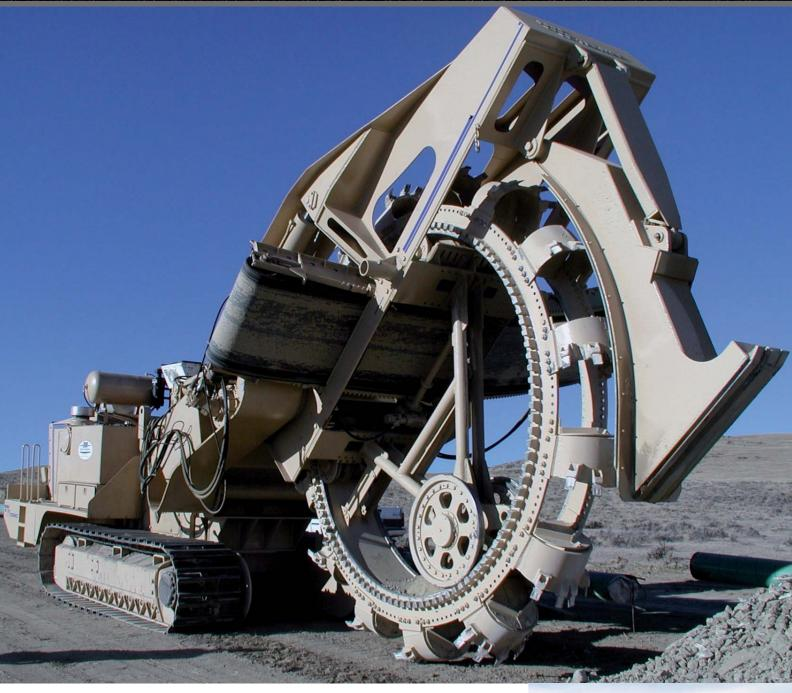
60 METRIC TON-CLASS BUCKET WHEEL TRENCHER FOR MID TO BIG SIZE PIPELINES AND UTILITIES EXCAVATION IN "DIRT" AND LIGHT ROCKY SOILS; THE 1175XHD MODEL IS AS A HIGH-PRODUCTIVITY MACHINE THAT CAN BE EQUIPPED WITH CONICAL OR SPADE TOOLS TO ENSURE THE MAXIMUM PRODUCTIVITY ACCORDING TO THE DIFFERENT GROUND CONDITIONS.
