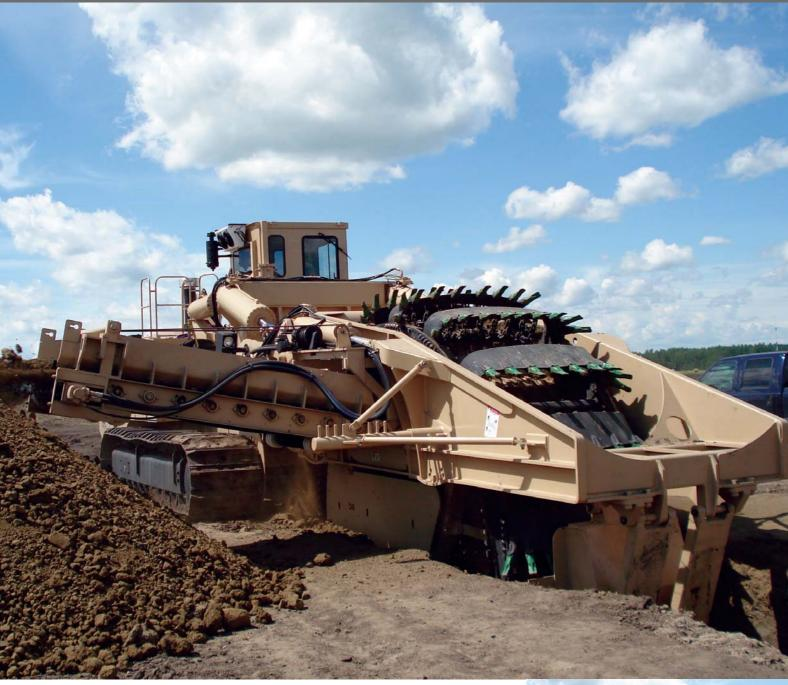
Tesmec's largest Bucket Wheel is conceived as a high-productivity machine for big diameter pipelines and utilities projects in "dirt" and light rocky soils. Its buckets can be equipped with conical or spade tools to ensure the maximum productivity according to the different ground conditions. No other trencher machine can grant such productivity in terms of linear meters per hour (foot per minute).
