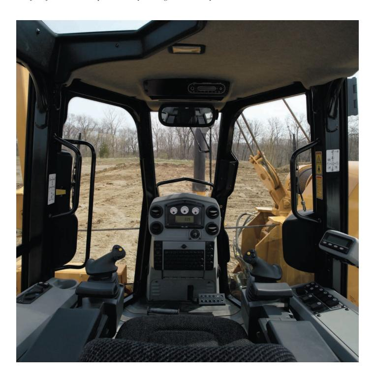
**Operator Station.** The operator station features an ergonomic layout emphasizing simplicity, ease of use and comfort. Standard air conditioning with enclosed cab, generous legroom and superior visibility allow the operator to focus on the job. With more glass area, the operator station provides a clear view to the surrounding work site.
