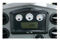
Instrument Cluster. The compact instrument cluster keeps the operator aware of all vital machine functions. The advanced monitoring system tracks machine operating conditions and informs the operator of impending problems. The monitoring system includes:
