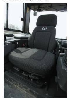
Air suspended seat. The Caterpillar C500 Comfort air suspended seat is available in cloth or vinyl and is fully adjustable, for maximum operator comfort. A standard lumbar adjustment provides excellent lower back support. For comfortable operation in cold weather, a heated cloth seat is available.
