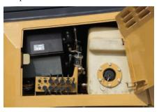
**Grouped Pressure Taps.** Pressure taps allow for quick measure and troubleshooting of the hydraulic system. These pressure taps are all located in the left service access door, and are accessible from ground level.
