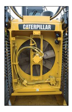
The engine radiator, Air To Air After Cooler (ATAAC), and hydraulic oil cooler are packaged in a single plane. Aluminum bar plate construction provides durability and allows for higher heat transfer and superior corrosion resistance. The standard cores feature 6 fins per inch to allow debris to pass through and reduce plugging concerns.
