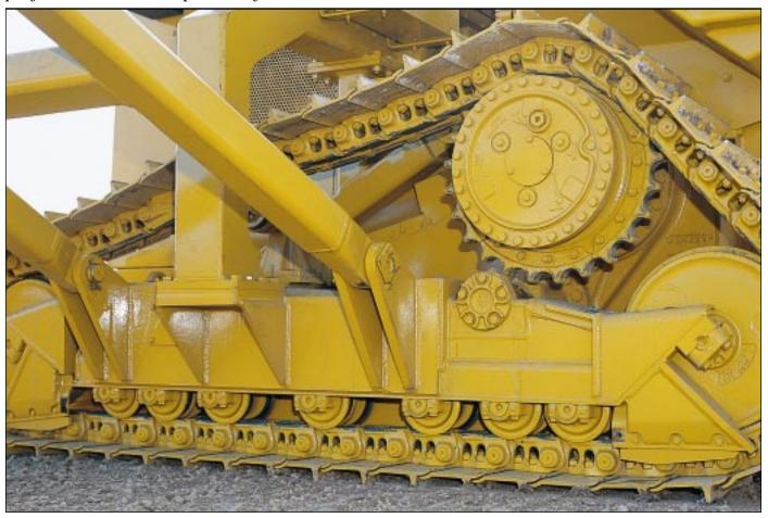
Final drives and associated power train components are raised above the work area, isolating them from ground-induced impact loads, as well as pipelayer loads, extending power train component life.
