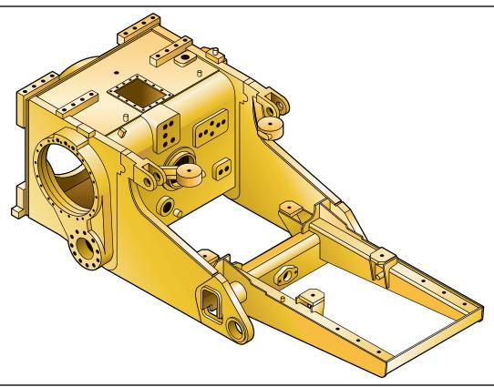
**High strength steel mainframe.** The 561M mainframe absorbs high impact shock loads and twisting forces.
