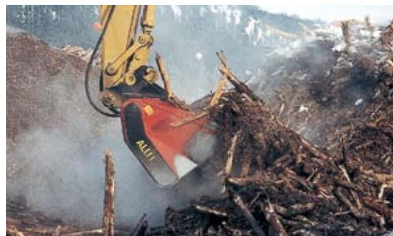
7. ALLU separates the fine from oversized materials.
